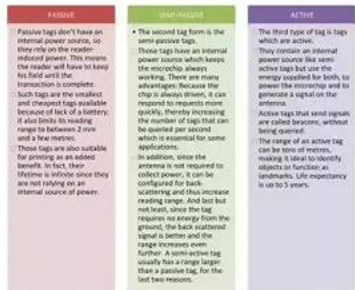
Figure 3: Types of RFID Tags and their working respectively.
