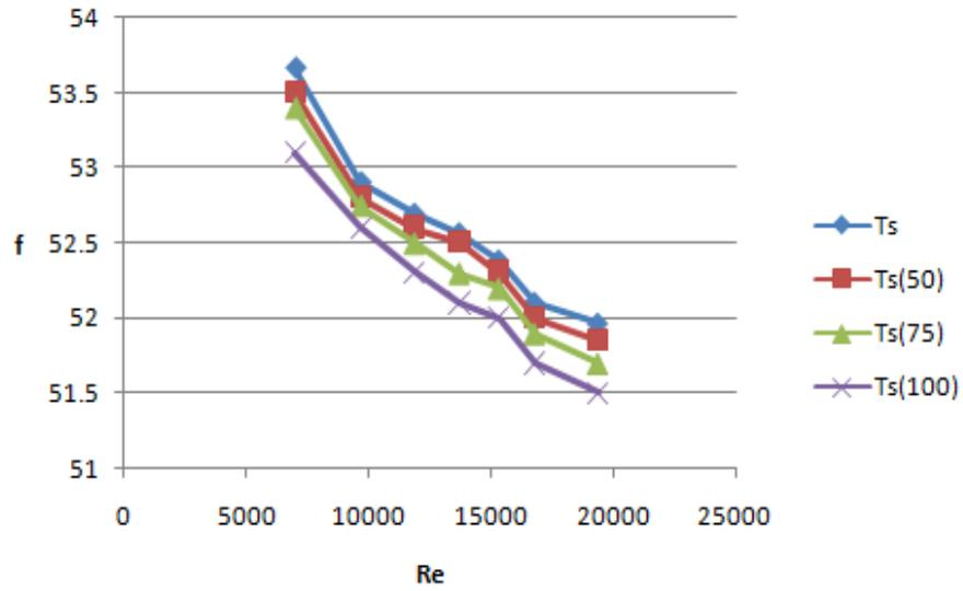
**Fig.12** Variation of Friction Factor Vs Reynolds No. for different fin height and its comparison with plate without fin
