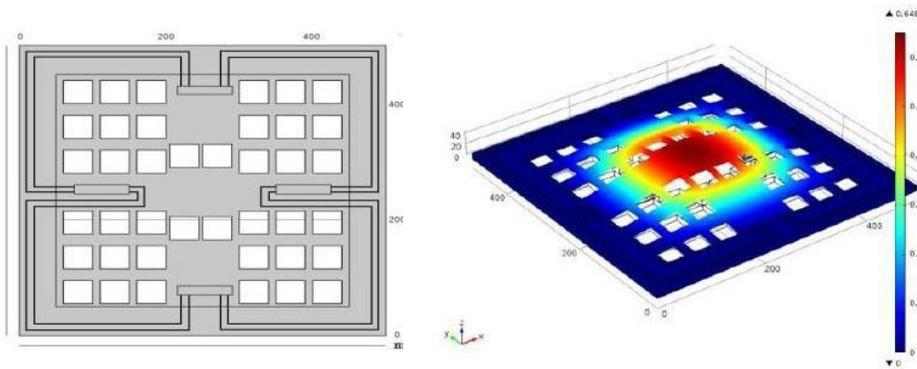
Figure 3 Perforated diaphragm design and stress level [17].
