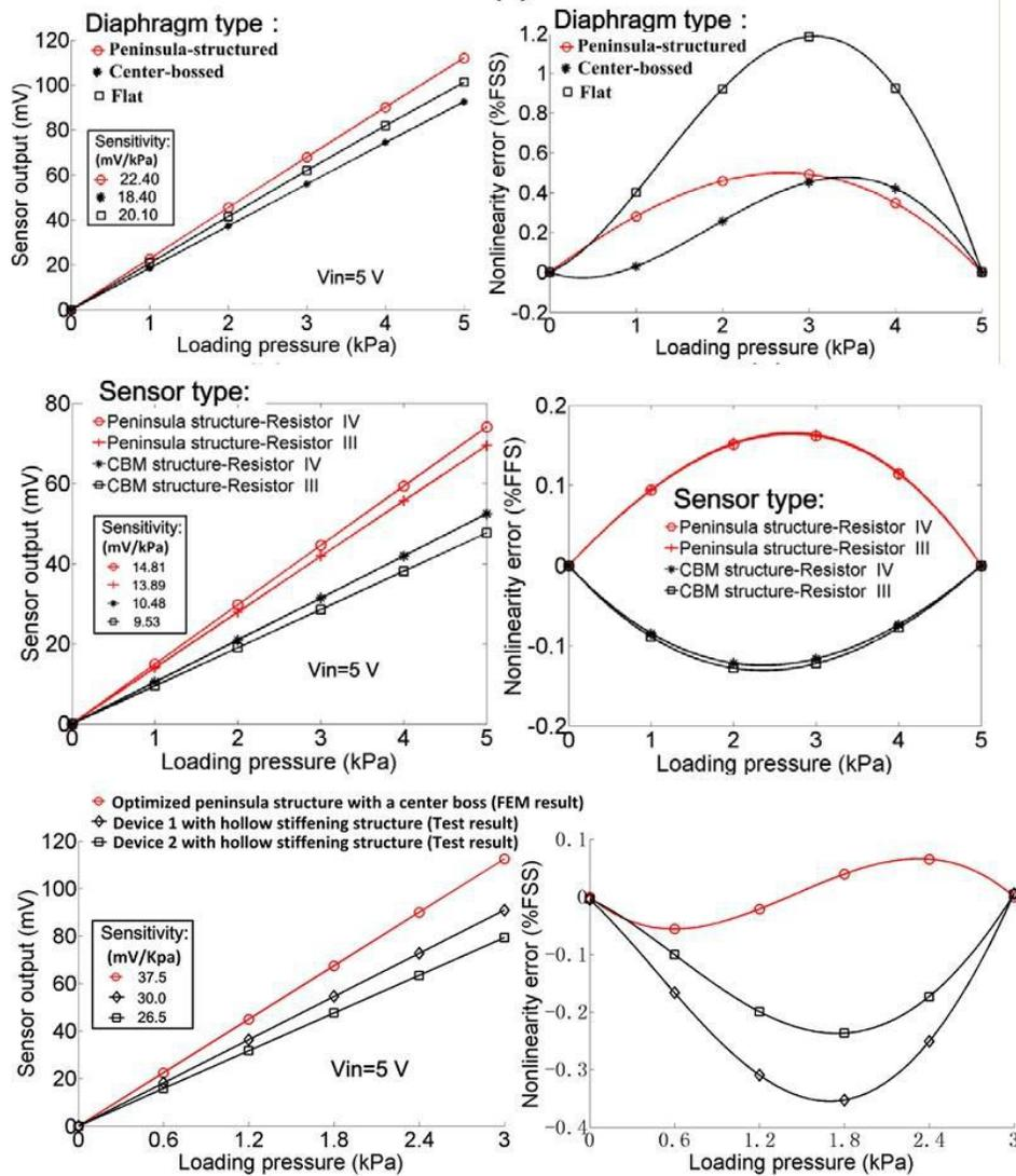
Figure 4 Comparison between center-bossed, CBM, hollow stiffening, and flat diaphragm structure [22].
