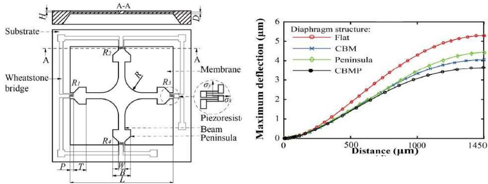
Figure 8 Crossed Beam Membrane Peninsula structure and comparison graph for membrane deflection.
