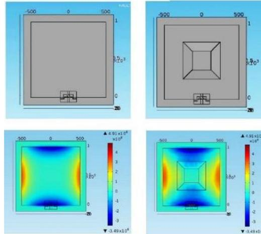
Figure 2 Increment in the stress level due to inner diaphragm structure as compare to Simple square diaphragm [15].
