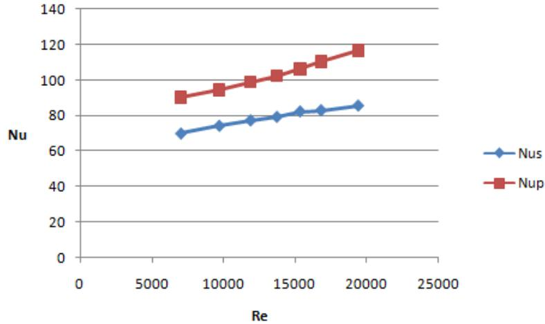
**Fig.6** Comparison of Nusselt no. vs Reynolds no. for  $C/H = 1, S_y/D = 1.2$
