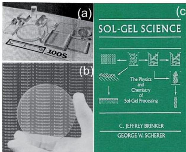
**Figure – 8.** a & b Illustrations of the earliest silica monoliths produced using sol-gel. c) The book cover for "Sol-Gel Science." Permitted adaptation. [159,169] Copyright Elsevier,1990.
