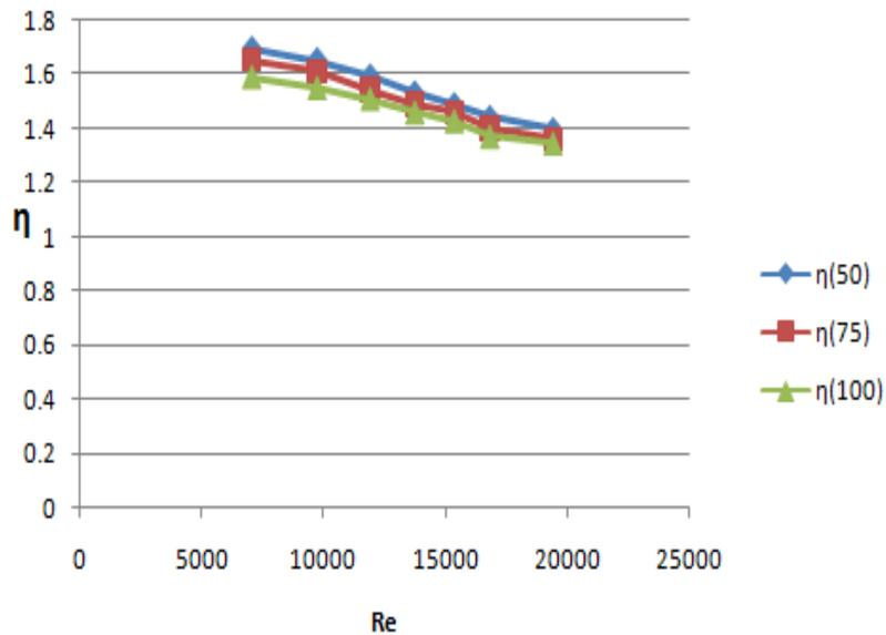
**Fig.13** Variation of Enhancement efficiency( $\eta$ ) Vs Re & its comparison for different fin height
