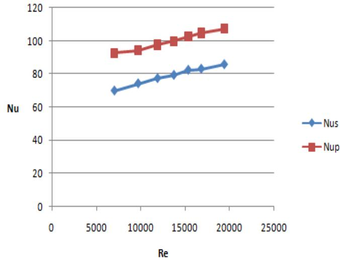
Fig.10 Comparison of Nusselt no. vs Reynolds no.  $C/H = 0.33$ ,  $S_y/D = 1.8$
