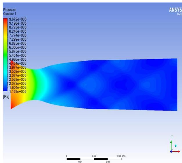
**Fig.4** Pressure contour with expansion wave
