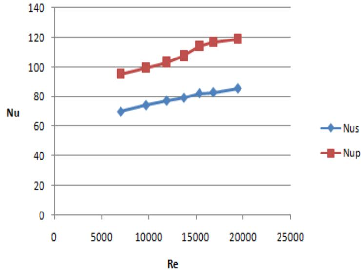
Fig.8 Comparison of Nusselt no. vs Reynolds no. for  $C/H = 0.33$ ,  $S_y/D = 1.2$
