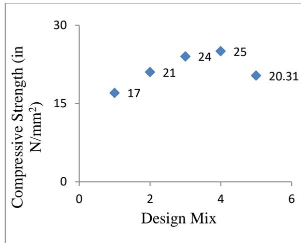
Fig: 4 Compressive strength of concrete at 14 days
