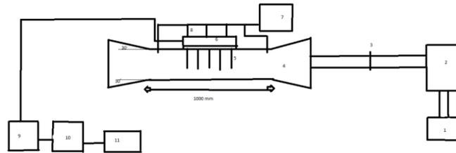
**Fig1.** 1-Moter, 2-Blower, 3-Orifice, 4-Duct, 5-Fins, 6-Heater, 7-Digital Temperature Indicator, 8-Thermocouples, 9-Ameter, 10-Voltmeter, 11-Power Supply
