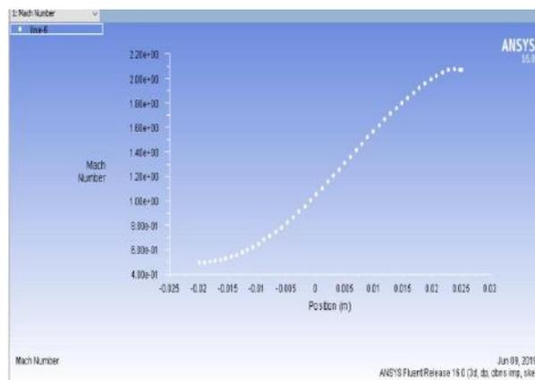
Fig.6 Variation of Mach No along the Nozzle
