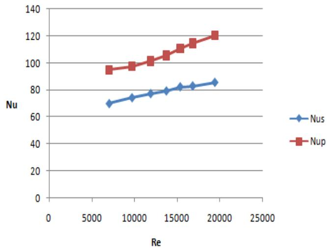
Fig.9 Comparison of Nusselt no. vs Reynolds no.  $C/H = 0.0$ ,  $S_y/D = 1.8$
