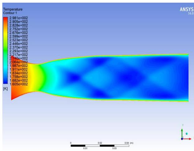
Fig 5 Temperature contour with expansion wave
