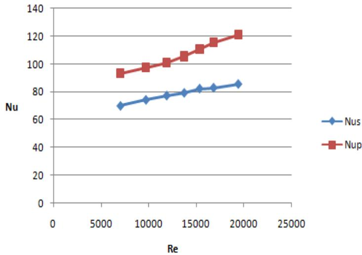
**Fig.7** Comparison of Nusselt no. vs Reynolds no. for  $C/H = 0, S_y/D = 1.2$
