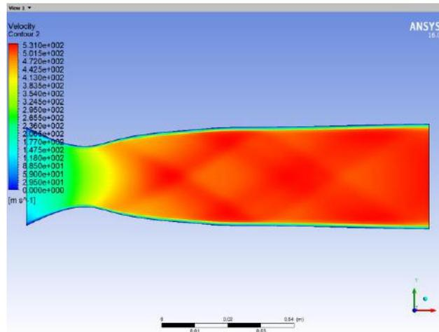
**Fig.3** Velocity contour with expansion wave
