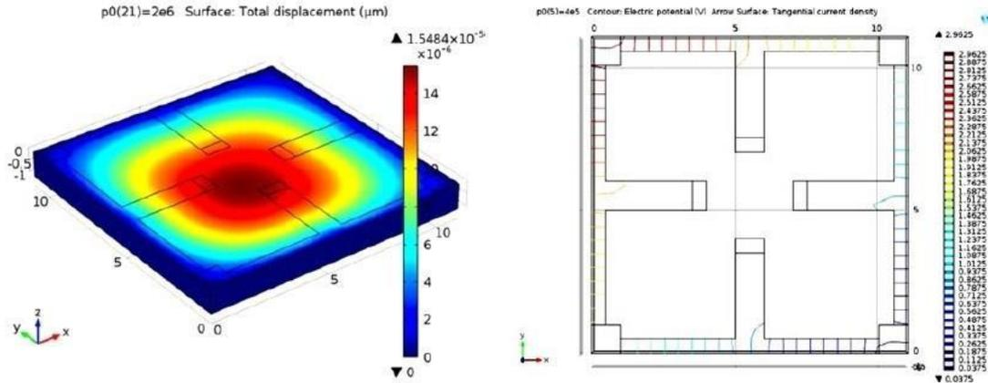
Figure 1 (a) Maximum deflection at Mid-point (b) Voltage distribution as per applied pressure.
