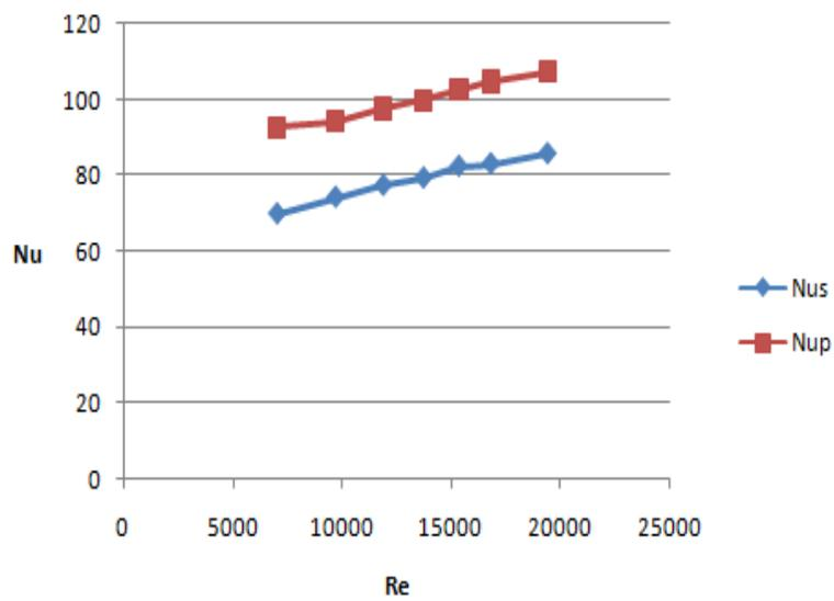
Fig. 11 Comparison of Nusselt no. vs Reynolds no.  $C/H = 1$ ,  $S_y/D = 1.8$
