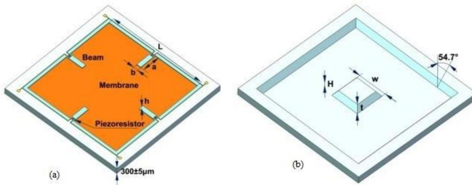
Figure 7 Four Beams Bossed Membrane (FBBM) structure.
