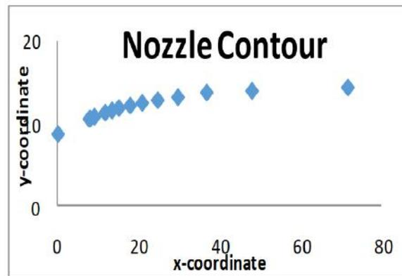
**Fig.1** Divergent section of Nozzle
