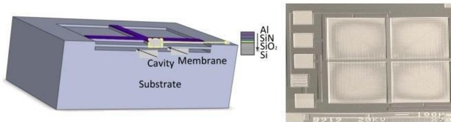
Figure 6 Four membranes crossed the beam structure.
