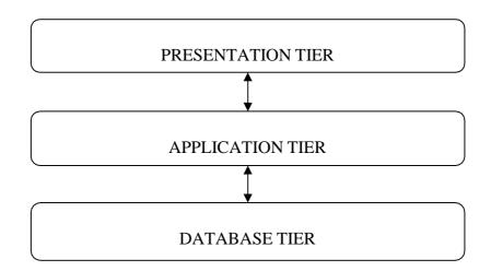
The DATABASE TIER has the database along with the query processing language. This is where all the table and relationship definitions are, also constraint on data access etc are also applied here.
